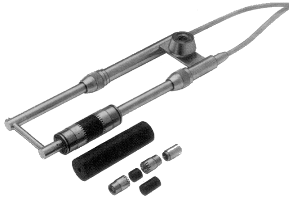
Figure 2-6: One dimensional sound intensity probe of Brüel & Kjær, consisting of two cylindrical pressure microphones, placed 'face to face', based on the p-p principle.
